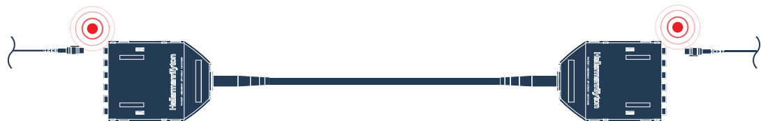
RapidNet MTP VHD direct termination with 2 mated pairs , a total of 1dB connector loss
