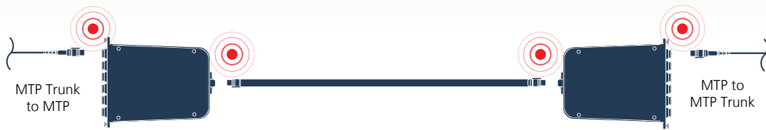
MTP to MTP trunk design required with 4 mated pairs , a total of 2dB connector loss
